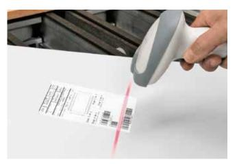
**No dead times:** the barcode reader lets you load the machining program automatically by simply scanning the
