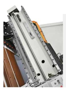
**Highly precise and fast movements:** all the machining units are driven by brushless motors, sliding along prismatic guides with recirculating balls supports. **The displacement** along X, Y, and Z is granted through highly precise recirculating balls screws.
