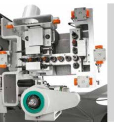
**Complete equipment of the machining unit:** drilling head for vertical and horizontal holes, blade for grooves along X axis and routing motor up to 5.5 kW at 18000 RPM.
