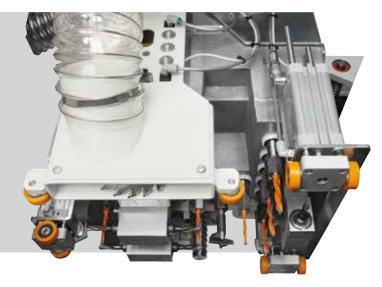
**Very short machining cycles** and **zero dead times** for set-up operations; the drilling head with 18 independent spindles (12 vertical, 4 horizontal along X axis, 2 horizontal along Y axis) and blade along X axis cover the whole surface of the panel to be machined: • length from 200 to 3050 mm
