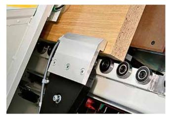
Maximum piece stability and high machining quality, with the mobile clamp with floating opening that does not require any adjustment and the Bakelite non-scratch table that guarantees high machining quality also for panels with delicate surfaces. Zero imprecision in horizontal drilling thanks to pressure devices.
